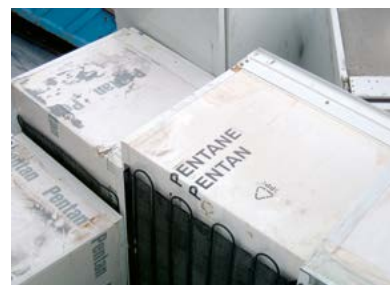
Even CFC-free refrigerators have to be specially treated.
